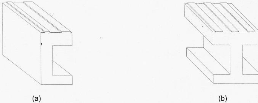
Figure 6 Typical specimens for hollow bricks: (a) shell, channel or U specimen; (b) web or I specimen
