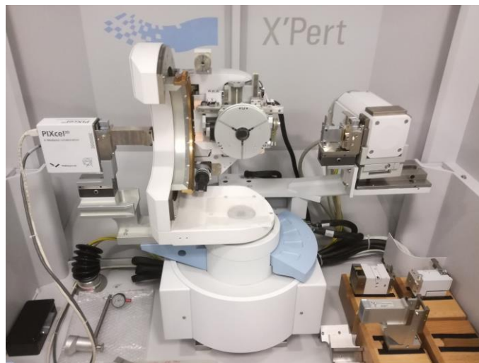
Figure 18 – X'Pert PRO PANalytical XRD equipment.
