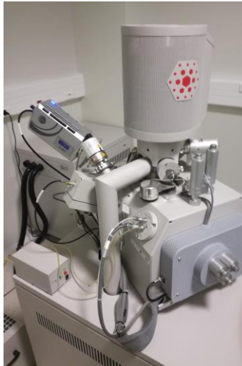
Figure 17 – SEM equipment Quanta FEG 650.
