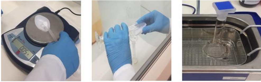
Figure 68 – Powder measurement (left). Mixing the powder with deionized water (middle). Thiourea in the ultra-sound (right).
