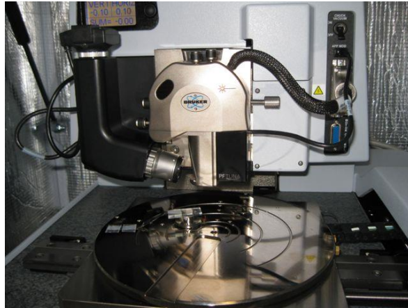
Figure 14 – AFM equipment, Bruker-Dimension Icon.
