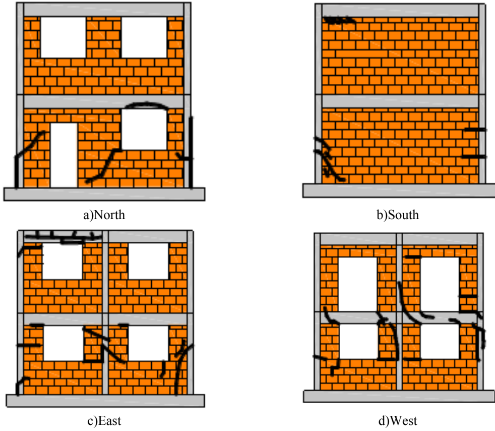
Fig. 15 Experimental crack propagation at stage 3 corresponding to 100% of the earthquake load (Leite, 2014)
