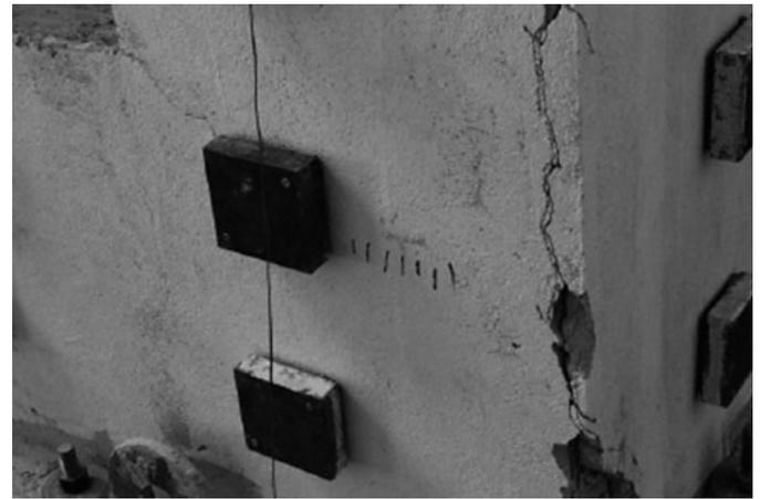
Fig. 16. Damage to building model 3 after loading stage 3
