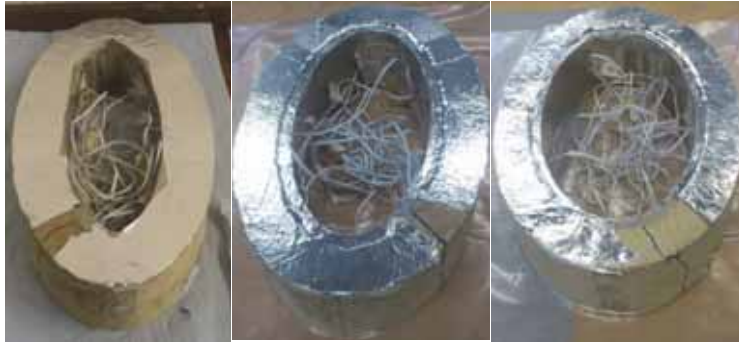
Figure 4: Crack positions in thin elliptical rings (left) a \times b = 150 \times 60 \text{ mm}^2 (centre) a \times b = 150 \times 75 \text{ mm}^2 (right) a \times b = 150 \times 100 \text{ mm}^2
