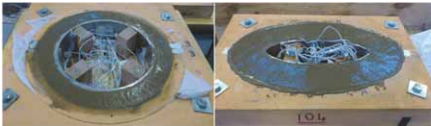
Figure 2: Thin circular ring (left) and thick elliptical ring (right) specimens in mould after concrete placement
