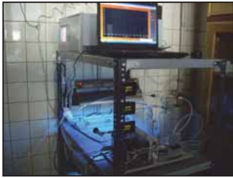
Figure 3 Test set-up according to ISO 221971-1:2007 [9] to determine the air purifying properties (NO x abatement) of the products.
