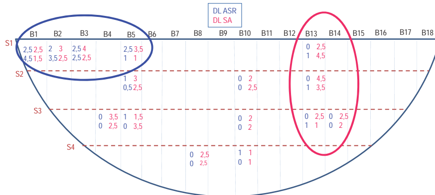
Figure 10. D1 structure damage Level (DL) graphic.
