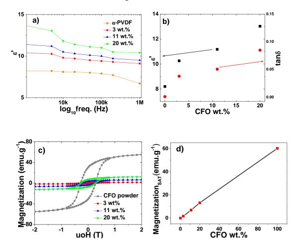
**Figure 1.** a) Frequency-dependent dielectric constant for CFO/PVDF nanocomposites and; b) variation of the dielectric constant (squares) and dielectric loss ( $tan\delta$  - circles) of the nanocomposites as a function of CFO content at room temperature for a
