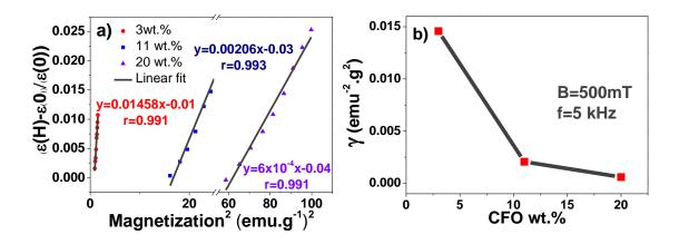
**Figure 4**. a) Variation of the dielectric constant versus  $(M)^2$  plot for the CFO/PVDF composites; b)  $\gamma$  as a function of the CFO content at 500 mT and 5 kHz.
