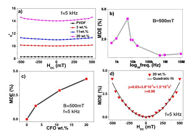
Figure 2. a) Dielectric constant as a function of the DC magnetic field at 5 kHz; b) MDE(%) as a function of the frequency; c) MDE(%) as a function of the CFO content at 500 mT and 5 kHz; d) Parabolic curve fitting of the MDE(%) as a function of the DC magnetic field.
