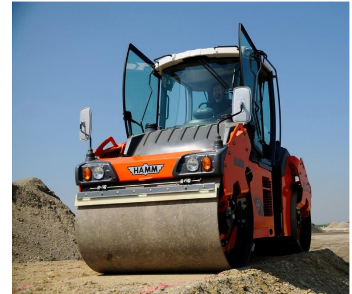
Compaction device: HAMM HD+ 90 VO tandem roller (ca. 9.8 t)
