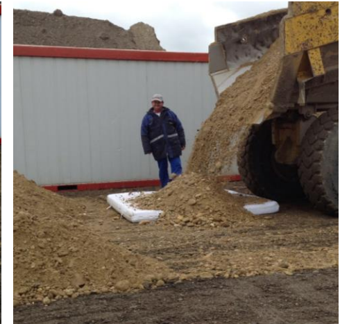
Installation of the artificial weak spot
