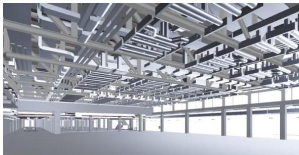
Figure 3.3: Rendering of the model of the proposed building: complex configuration of MEP equipment over steel trusses.
