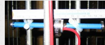
vibrating wire for (almost) measurement of \sigma_c / E(t)
