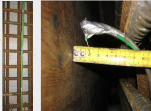
thermocouples in several material points for \Delta T
