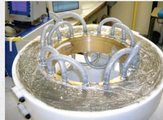
Ring test after casting
