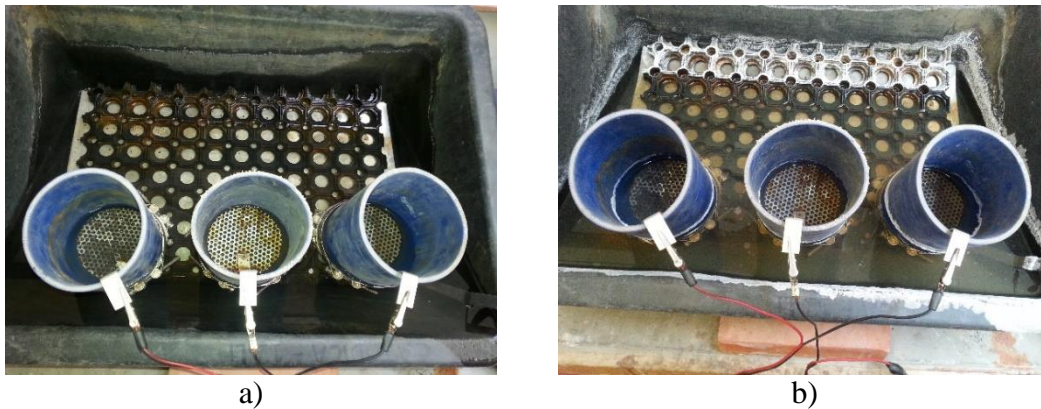
Figure 5: The cathodic solution at the beginning (a) and after 14 days in 60 V (b).
