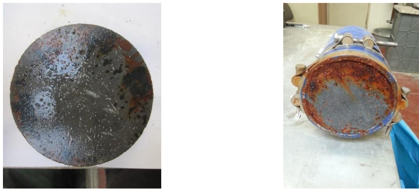
Figure 4: Corrosion of specimens' surface.
