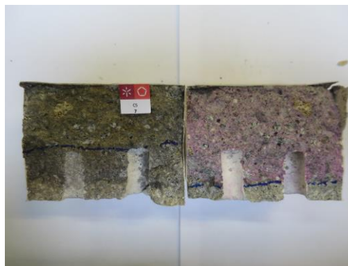
Figure 3: Chloride depth (left) and Carbonation depth (right) reached in group A.
