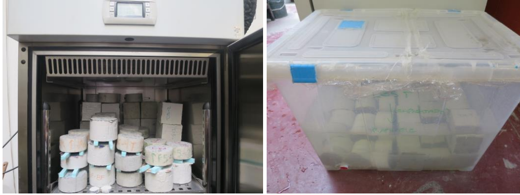
Figure 1: Combined action: Carbonation test (left) and Immersion test set-up (right).
