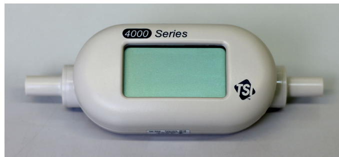
Figure 4.9: Mass flowmeter used in the rotameter calibration and in the variable flow setup
