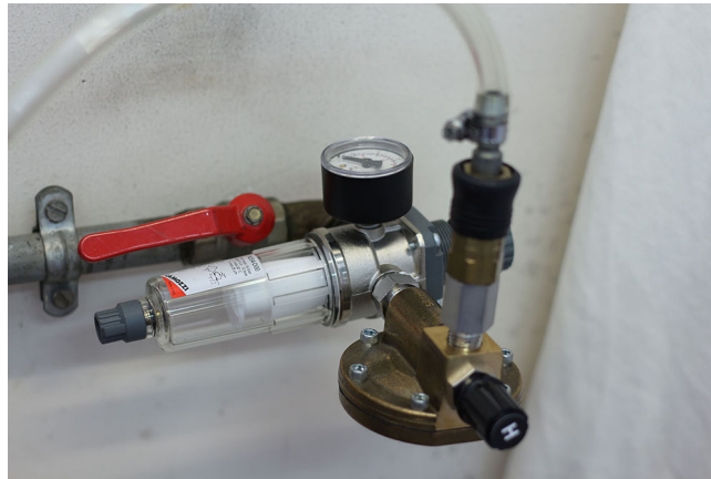
Figure 4.7: Air compressed source with the assembly of the pressure regulator and flow regulator
