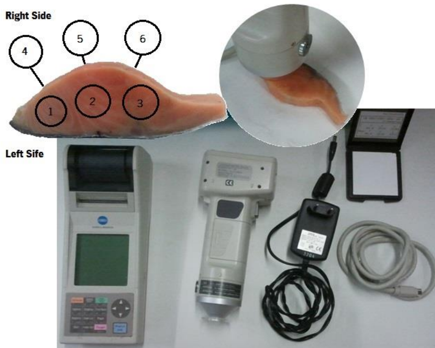
Figure 6-2 - Illustration of the methodology and equipment used in the measurement of the colour of salmon.
