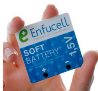
Figure 2.6: Enfucell's thin, flexible and ecofriendly “SoftBattery”
