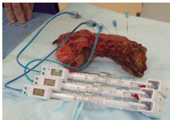
Figure 2.9. Test performed by Menkowitz et al. (2005). During the pressurization test, the structure was not confined or axially loaded.
