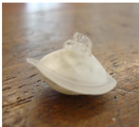
Figure 6.A.5. The rupture zone in the “Ravioli”, corresponding to the “normal plane” of the ring region.
