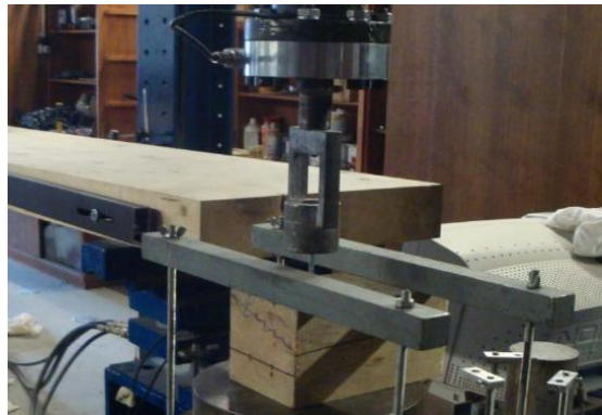
Figure 4: Setup used in laboratory for the withdrawal tests.
