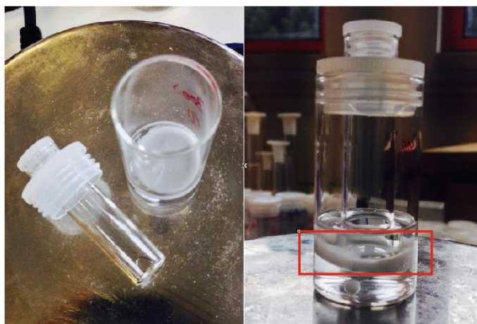
Figure 2.2: Disassembled (left) and assembled (right) modified glass vial used in drug release assays, with a submerged membrane (red rectangle).
