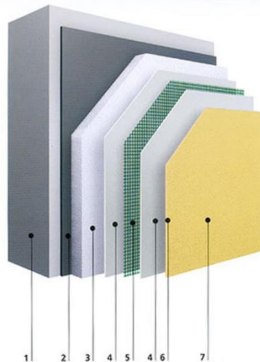
Figure 7 - ETICS system (1-Brick or thermal block; 2-Adhesive; 3-Thermal Insulation; 4-Reinforcement-mesh embedding; 5-Reinforcement mesh; 6-Primer; 7-Rendering mortar) (L37, 2014)
