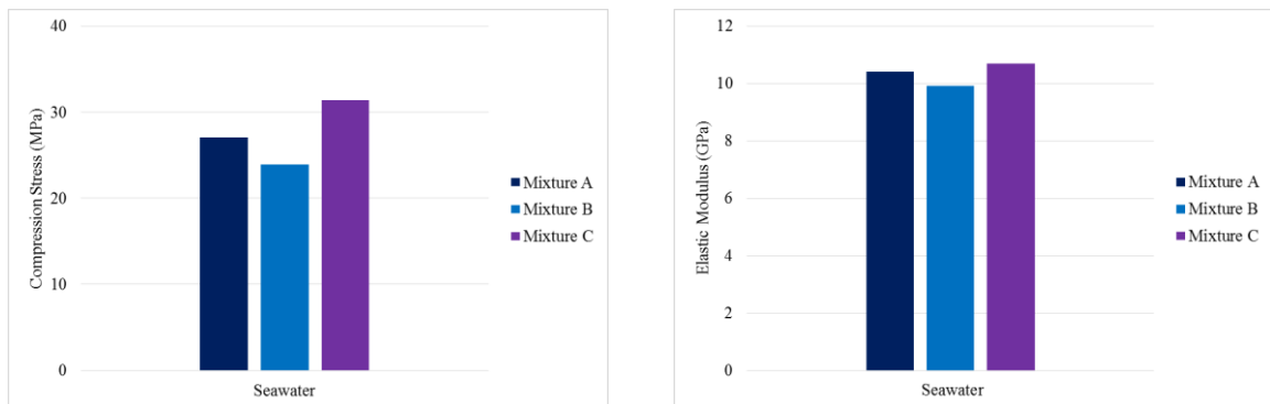
Figure 3.92- Compressive strength and elastic modulus obtained 14 days after curing in seawater.
