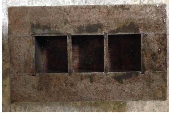
Figure 3.5-.Moulds used to cast the specimens for compression testing.
