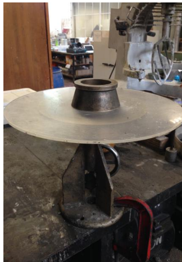
Figure 3.3- Setup used to perform the mini-slump test.
