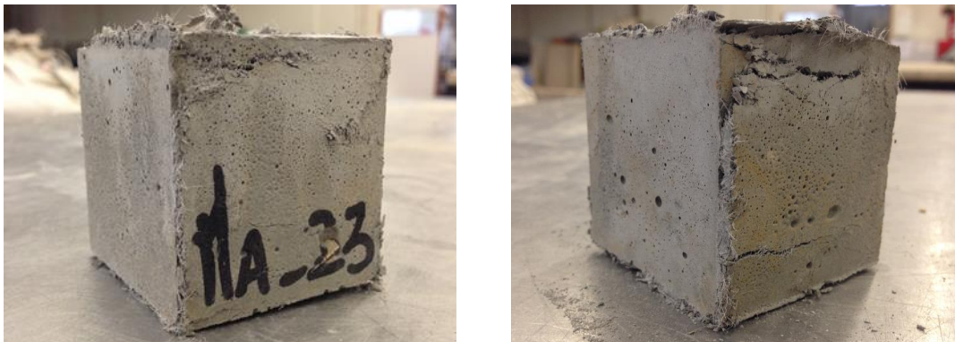
Figure 3.11- Example of a cubic specimen after testing.
