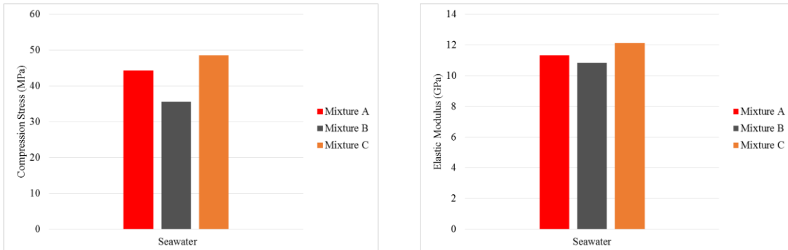
Figure 3.94- Maximum compressive stress and elastic modulus of different mixtures cured in seawater (28 days)
