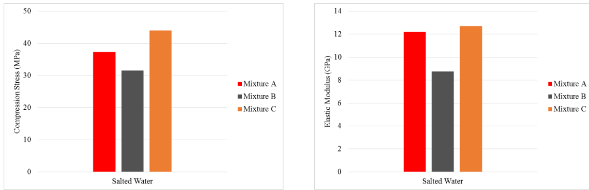
Figure 3.116- Maximum compressive stress and elasticity modulus of different mixtures cured in salted water (28 days)
