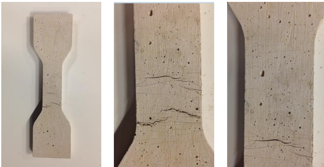
Figure 5. 18- Photos of GP_2.0_PVA_02 specimen after testing.
