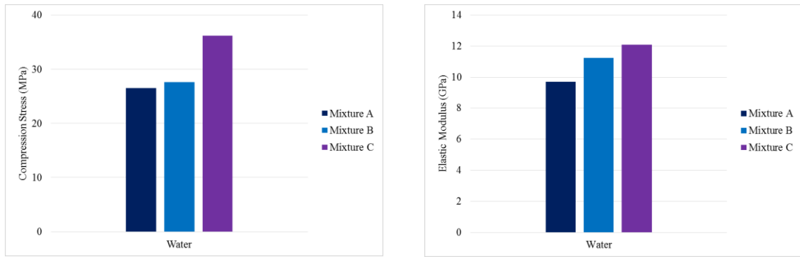
Figure 3.103- Compressive strength and elastic modulus for specimens cured in tap water for 14 days.
