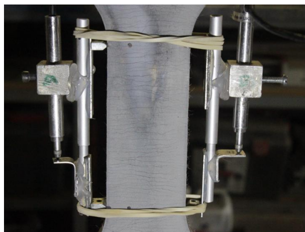
Figure 3. 31- Method used to measure the central displacement of the specimen
