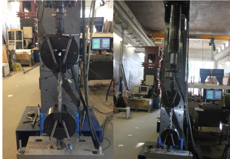
Figure 3. 30- Test setup used for the tensile tests
