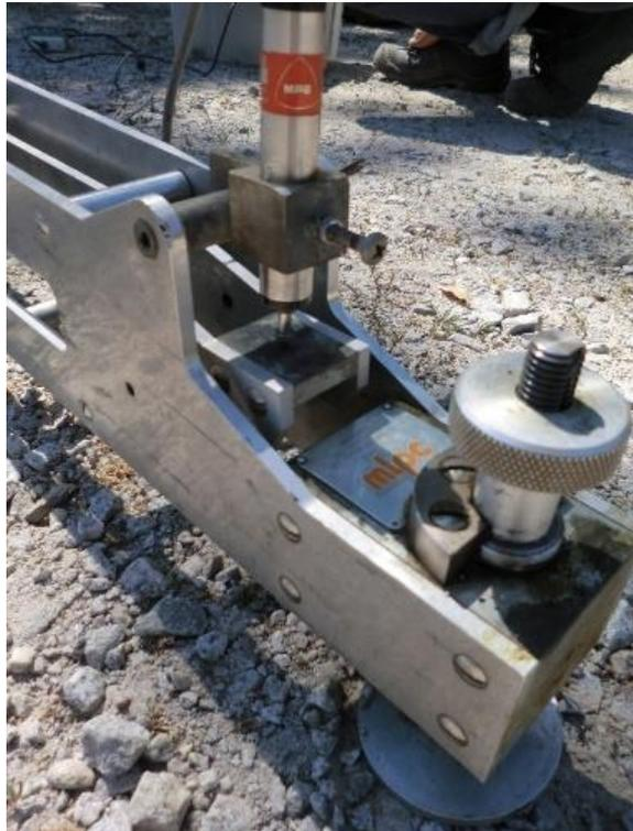
Figura 28 - LVDT (*Linear Variable Differential Transformer*)
