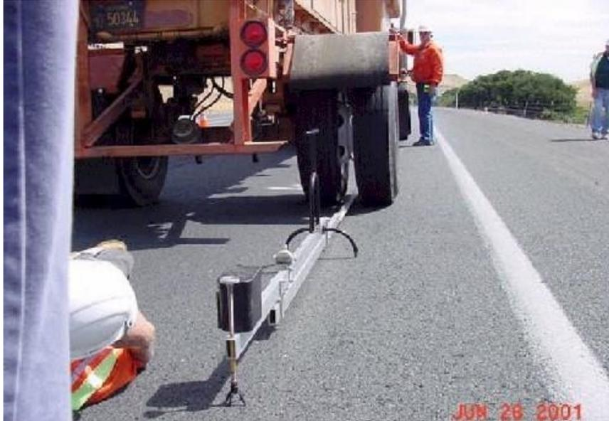
Figura 8 - Ensaio com Viga Benkelman (Pavement Interactive, 2010)
