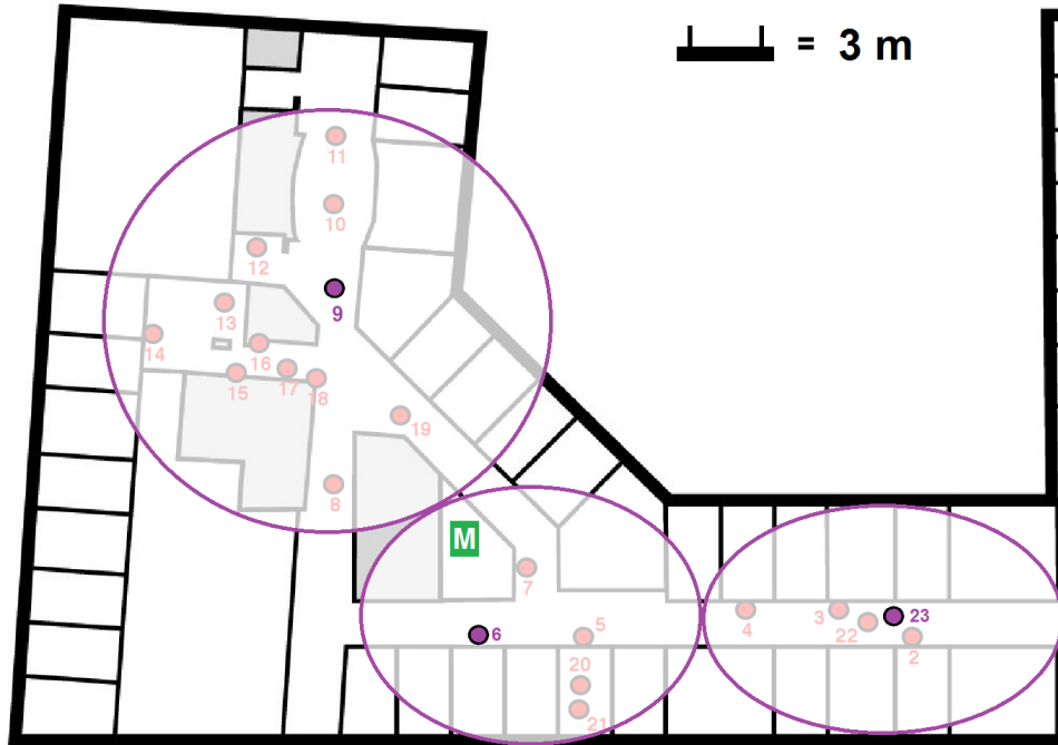
FIGURE 2.1: Testbed augmented with JamLab. Nodes 6, 9, and 23 are selected as HandyMotes, and take care of interference (re)generation in their respective cell, corresponding to the circled areas.
