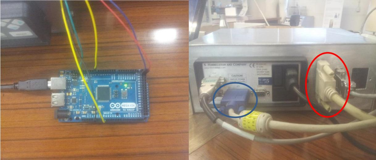
Figure 2 – Connection between Arduino and the motor driver (red) and the signal conditioner (blue)
