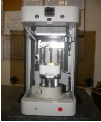
Figure 2.8 - Tribometer for friction and wear tests (Bruker, USA), courtesy of the Tribology Laboratory, UMinho
