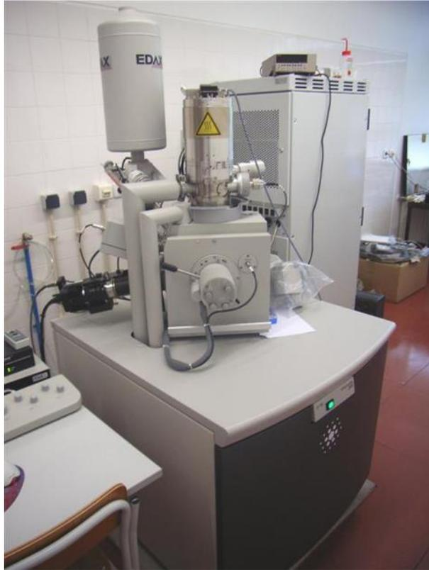
Figura 18 - NanoSEM – FEI Nova 200 (FEG/SEM).
