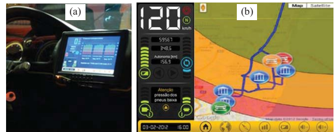
Fig. 3. Head unit prototype with mirror approach of the V2Anything App : (a) VEECO cockpit; (b) Application with route guidance to near charging points.
