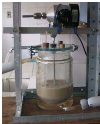
Figure 1. Bioreactor photo used in hydrolysis assays of manioc starch by amylases from maize malt.
