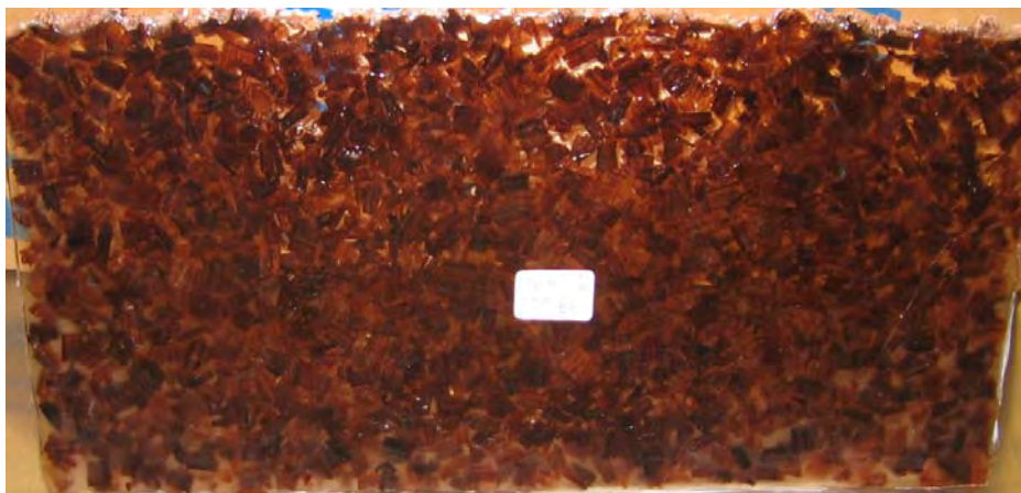
Figure 2. A typical plate of wood polymer composite, produced in this work (test #2 in the experimental design).
