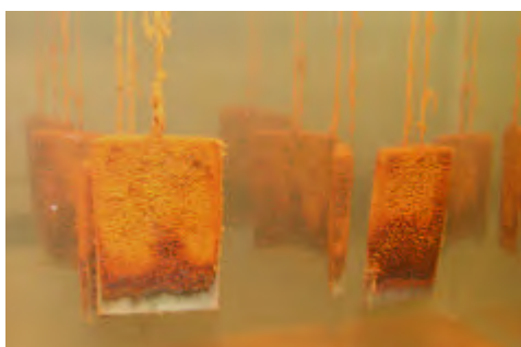
Figure 2 - Formation of biofilm in steel carbon AISI 1020 coupons after 45 days of exposition to the sea water.
