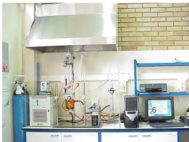
Figure 2 Bench scale set-up for preparing aqueous polyurethane dispersions.
