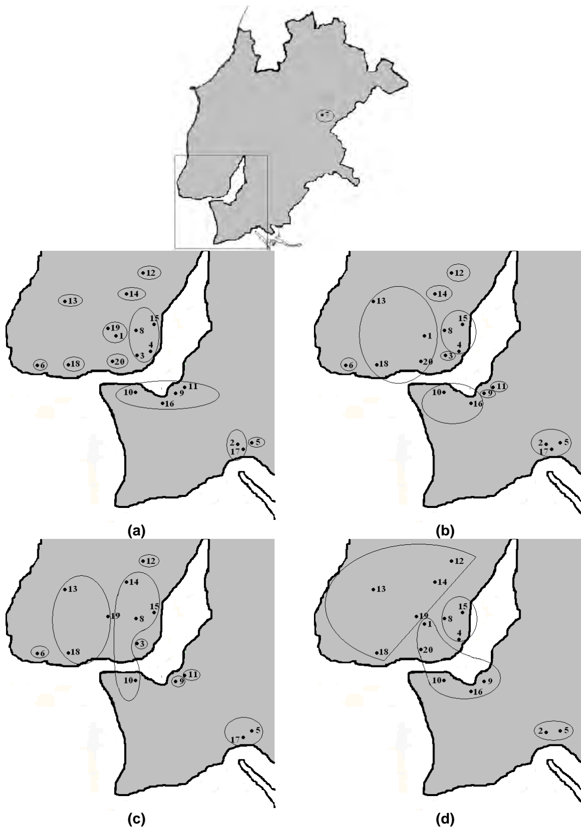
Figure 1. Location of monitoring sites and the PCA results using: (a) CO concentrations data (CO concentrations were not measured at S7 site); (b) NO 2 concentrations data (S19 site did not present 75% of the annual data); (c) PM 10 concentrations data (PM 10 concentrations were not measured at S2, S4 and S16 sites; S1 and S20 sites did not present 75% of the annual data); (d) O 3 concentrations data (O 3 concentrations were not measured at S3, S6, S11 and S17 sites).
