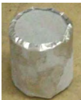
Figure 1. Synthetic unconsolidated sandstone plug
