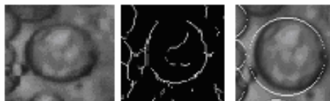
Figure 2: Original image, the edge detection and the detection of the drop using the Hough transform.
