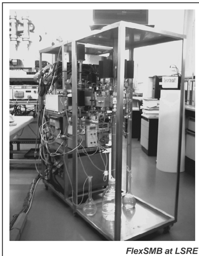
Figure 5 – Flexible SMB unit, the FlexSMB-LSRE.
