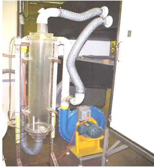
Figure 1 Fluidisation column connected to the heat pump dryer
