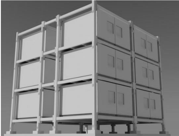
Figure 4: Scheme of the modular building, hereby considered only with the skeleton and modules. [Pedro Andrade]
