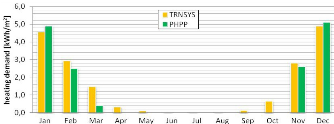
Figure 7. Comparison of monthly specific heat demand obtained by calculations in PHPP and TRNSYS.
