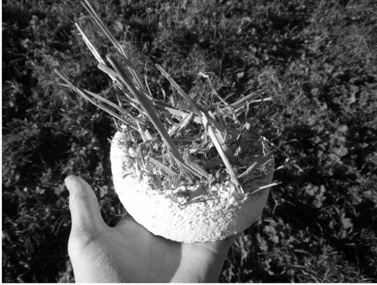
Figure 5. External render core removed from exposure test facility
