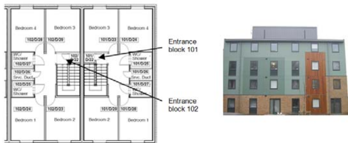
Figure 7. Location of monitoring sensors in the selected townhouses block (101 and 102).
