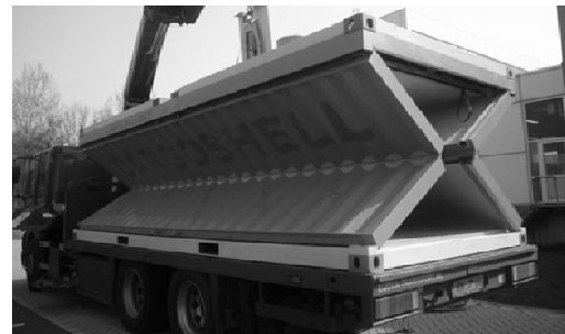
Figure 8. Disassembling load container for transportation. Source:
