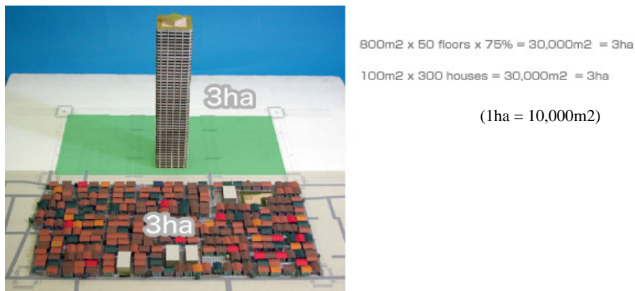
Figure 6. Efficiency of land use with super tall buildings in compact city (Mori, 2008)
