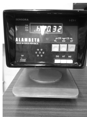
Figure 2: Alambeta equipment for thermal properties measurement.
