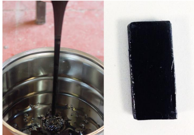
Figure 2-15 Bitumen 35/50 (left) in the liquid state at T > 60^\circ\text{C} and (right) in the semi-solid state at room temperature.
