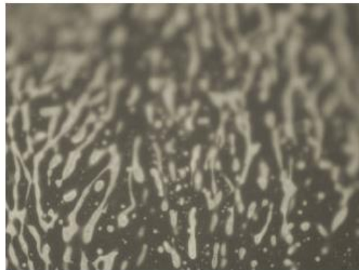
Figure 2-31 Example of a micrography of a sample (SBS PMB) without optical smoothness [42]
