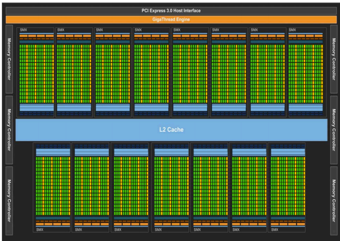
Figure 2.2: Diagram of the Kepler architecture (from NVidia documentation).
