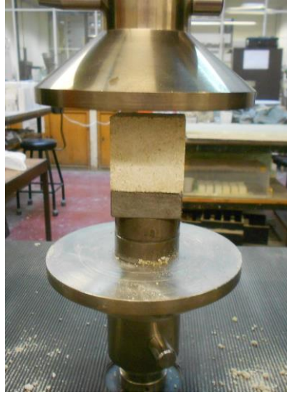
Figure 16: hydraulic press apparatus for compressive test (Meneghini, 2014).
