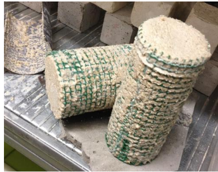
Figure 22: Cylindrical specimens after the tube removal, stored inside the standard chamber
