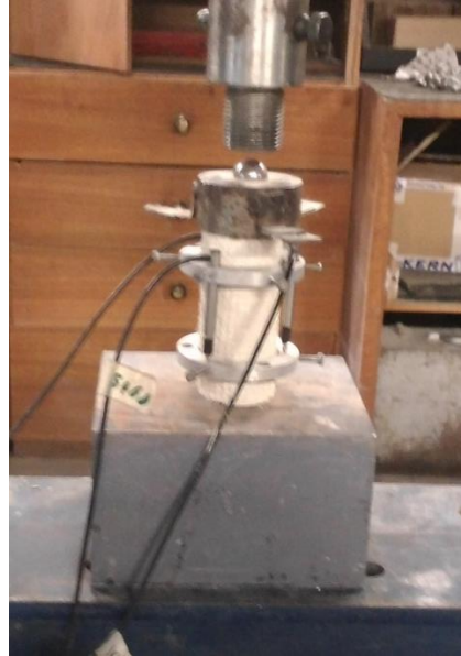
Figure 35: Experimental setting for the modulus of elasticity testing.
