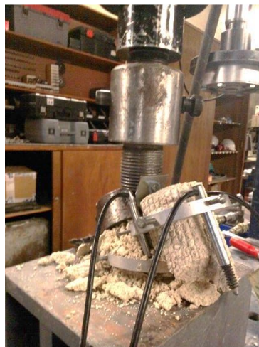
Figure 36: Damage in specimen EM_T20H90_1 on the first day of testing
