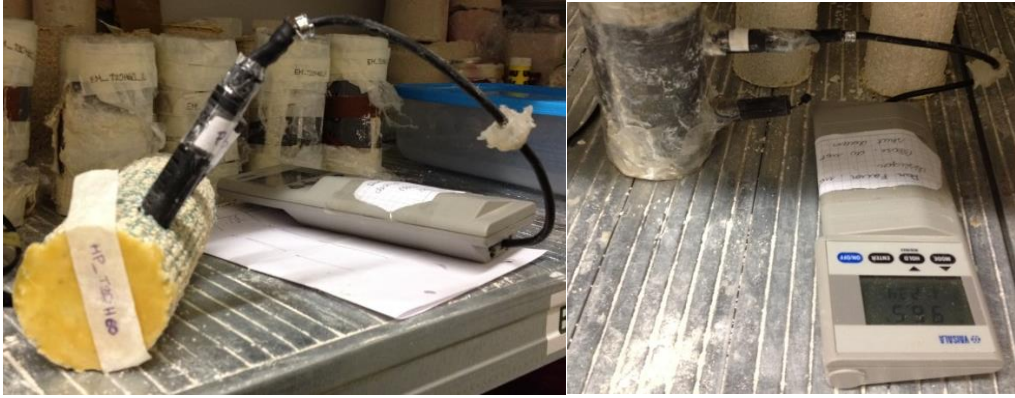
Figure 34: Measuring of humidity profiles in exposed and sealed specimens respectively.
