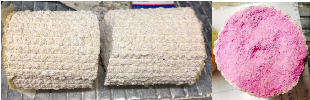
Figure 33: Section adopted for staining of the reused TGA cylindrical specimens
