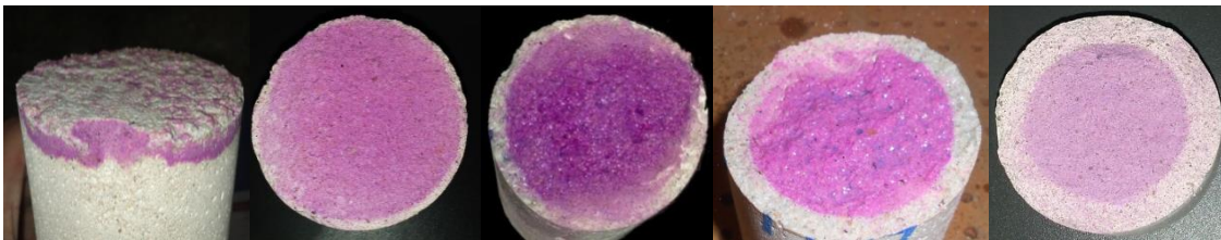
Figure 11: Horizontal section of stained specimens at 4,7,14 and 36 days of age, respectively. (Meneghini, 2014)
