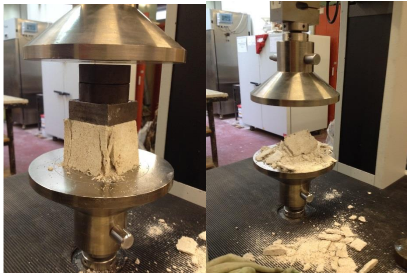
Figure 37: Pattern of failure of specimens stored in the wet chamber (left) and standard chamber (right)
