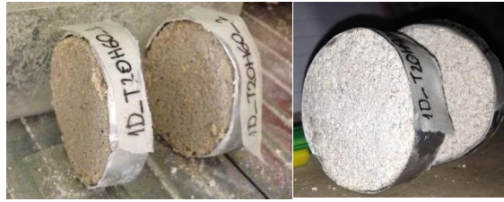
Figure 18: Disc specimens stored in the standard and wet chambers, respectively
