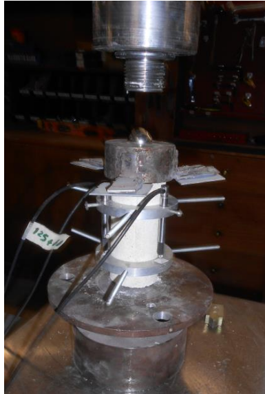
Figure 14: Setting of experimental testing apparatus on specimen.
