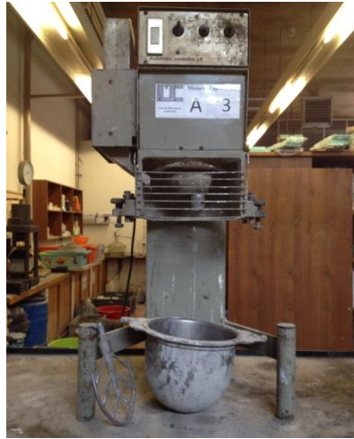
Figure 17: Mixer used in the mixture design
