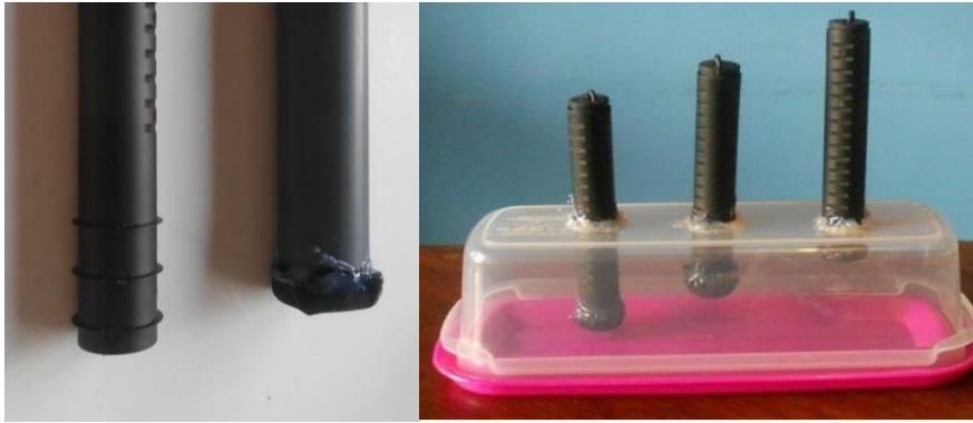
Figure 6: Vaisala sleeves and the mould apparatus for humidity profiles measurements (Meneghini, 2014)
