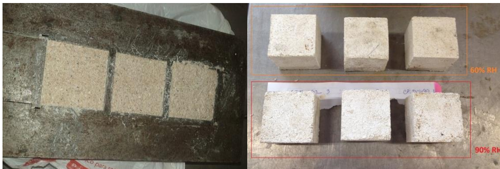
Figure 27: Mold sets used in the casting procedure and the demoulded cubic specimens
