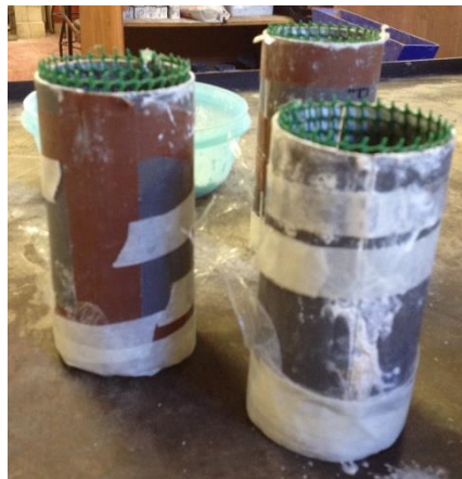
Figure 19: Mould system used in the casting of cylindrical specimens
