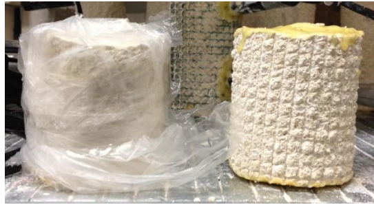
Figure 32: Specimen 3D_T20H60_5 after sectioning. The left piece is used in the 14 day testing, while the right one is saved for the next age of test.
