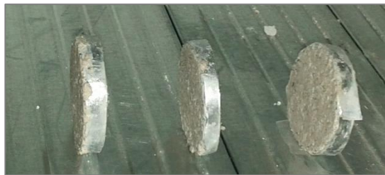
Figure 5: Disc-shaped specimens for TGA analysis (Meneghini, 2014)
