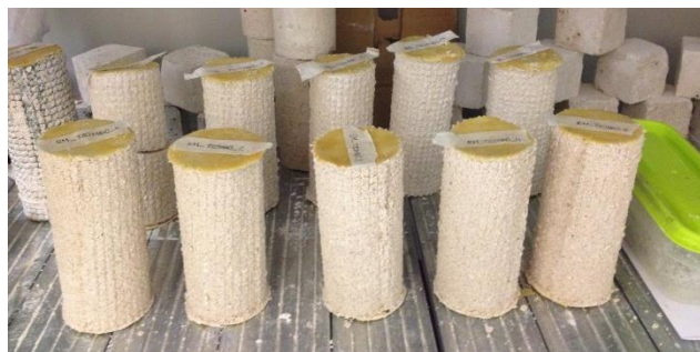
Figure 23: Demoulded cylindrical specimens storing position inside the standard chamber
