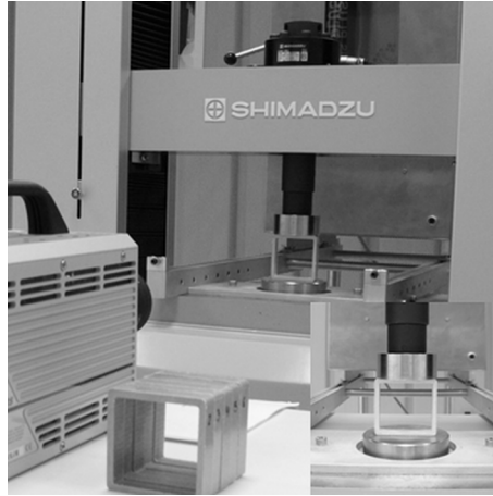
Figure 3.1.: Test set-up for lateral compression tests of pultruded box beam sections
