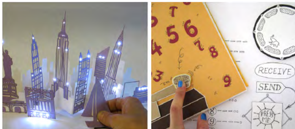
Figure 4-5 The Electronic Popables (Qi & Buechley, 2010) (left), and the Telescrapbooks (Freed et al., 2011) (right).
