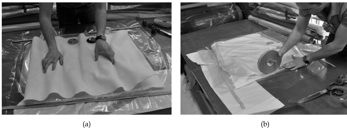
Figure 6.11. Wrapping of the laminates with breather material (a) and closing of the bag with mastic sealant (b).
