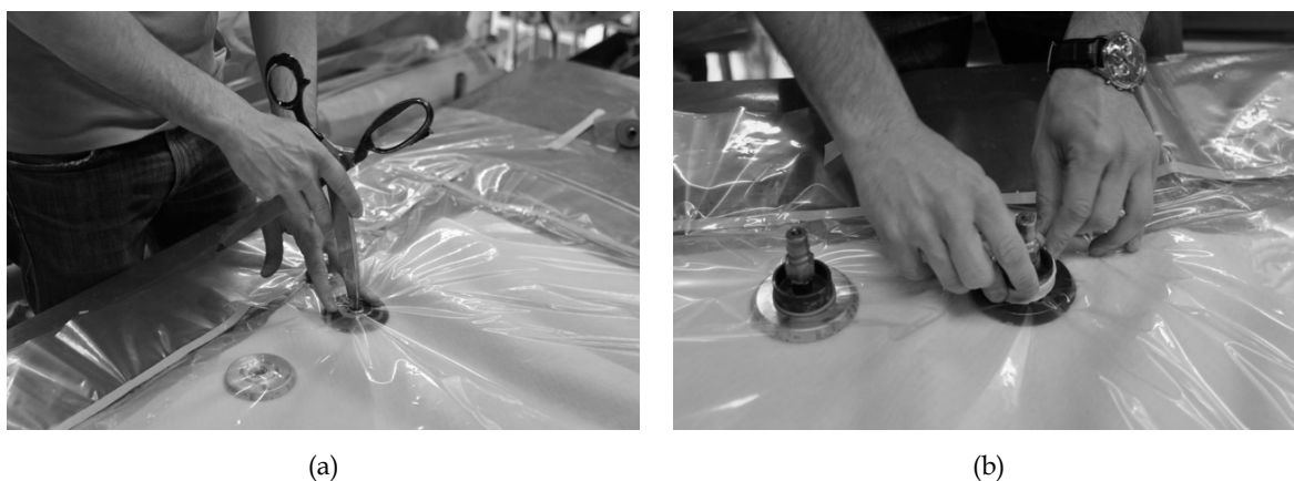
Figure 6.12. Perforation of the vacuum bag (a) and sealing of the pump valve connection (b)
