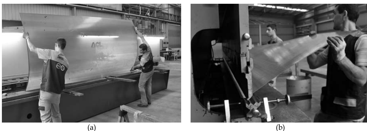
Figure 10.16. Cutting of the steel plates with a shear machine (a) and bending with a brake machine (b).
