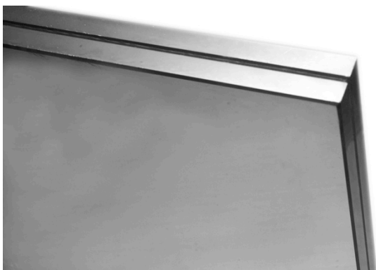
Figure 4.2. Sample of a laminated glass unit.
