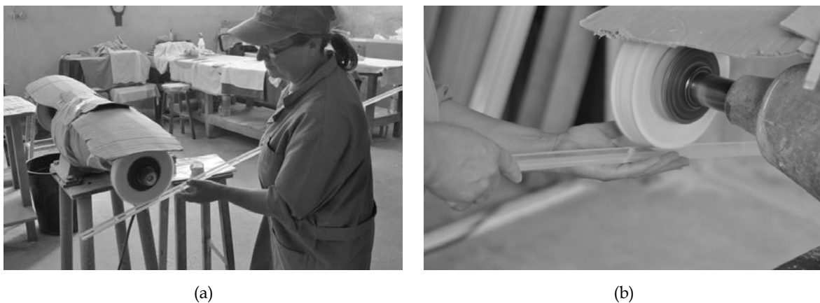
Figure 10.15. Polishing process with rotating disc machine (a) and close-up view of the process (b).
