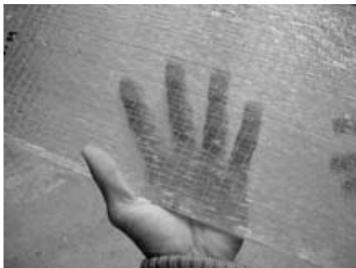
Figure 4.6. GFRP reinforced glass investigated by Speranzini et al.
