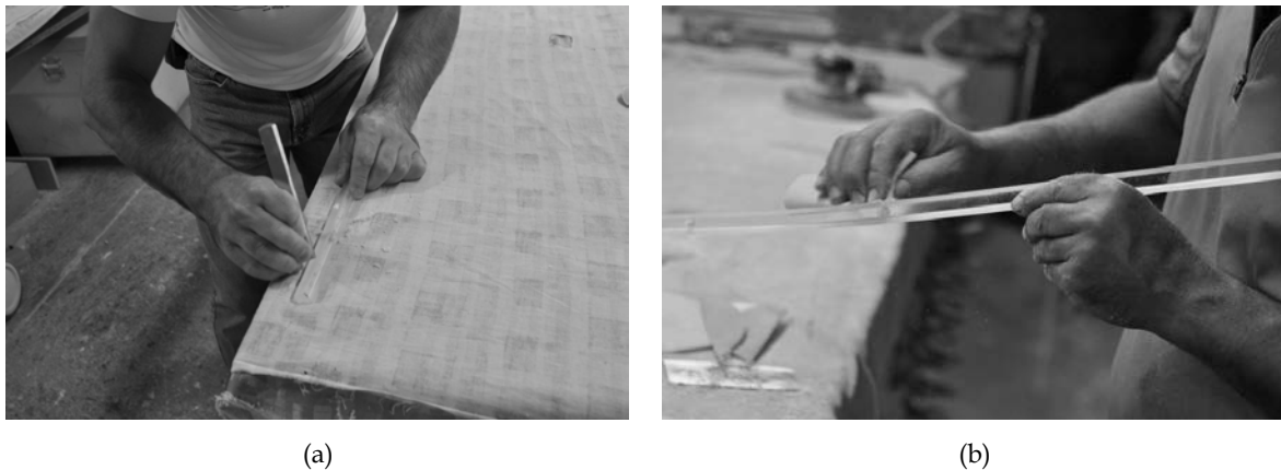
Figure 10.14. Manual grinding of the acrylic bar edges (a) and manual sanding of the surface (b).
