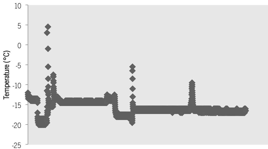
Figure A.12. Air temperature of freezing chamber registered every 10 minutes by a data logger during frozen storage.
