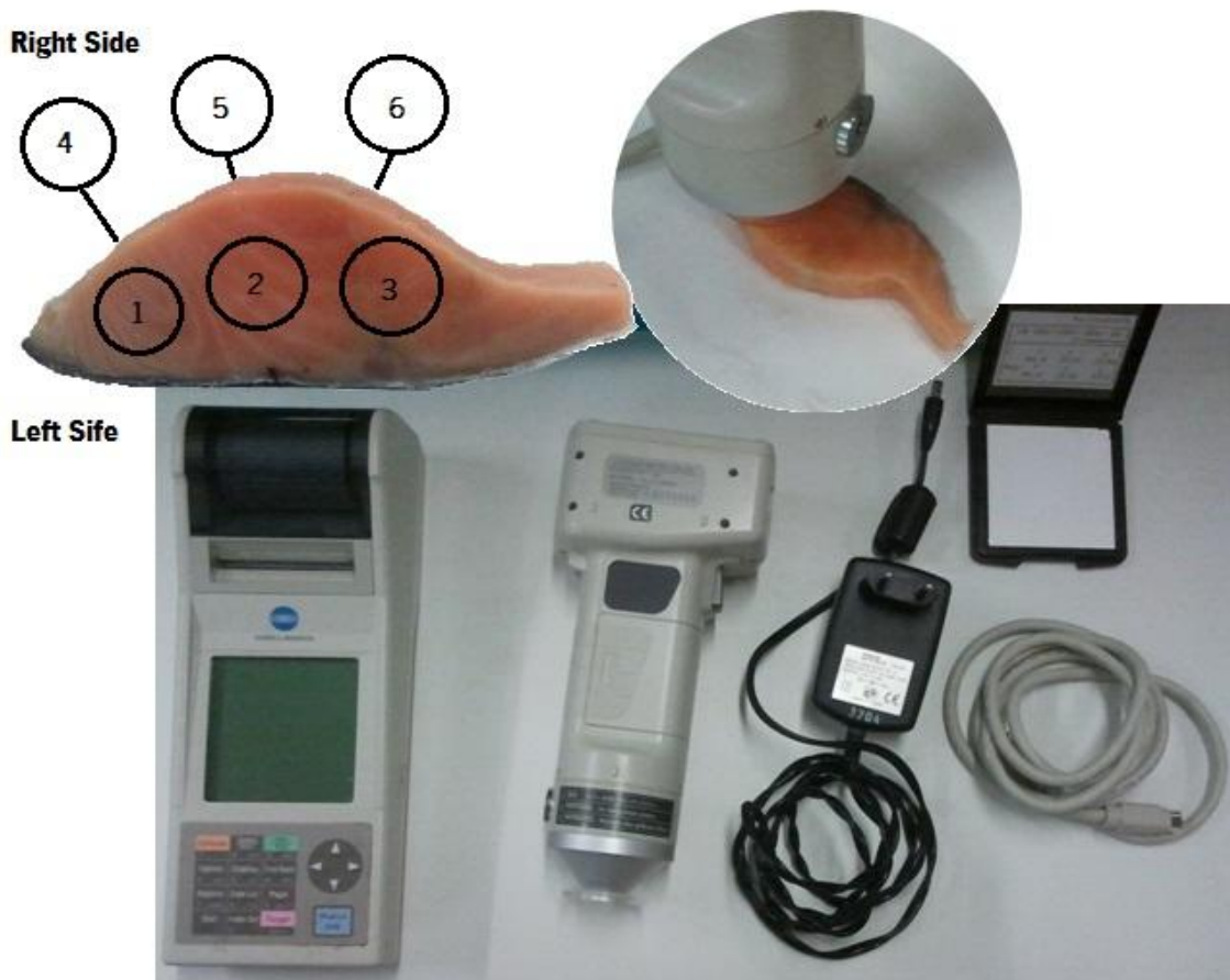
Figure 3.7. Illustration of the methodology and equipment used in the measurement of the color of salmon.
