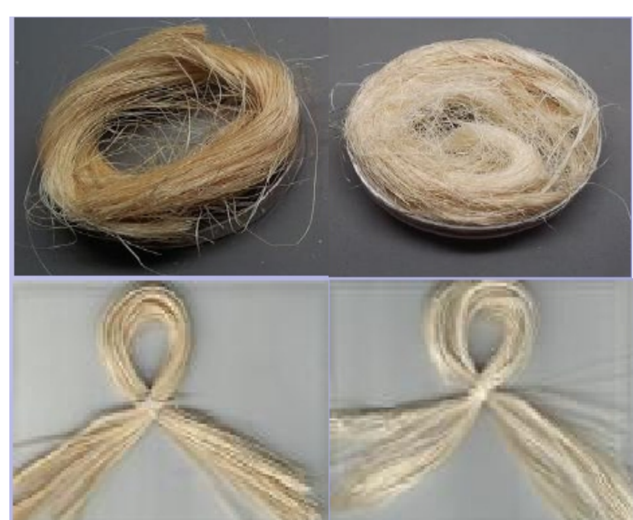
Curaua (above) and banana fibres extracted, before and after bleaching.
