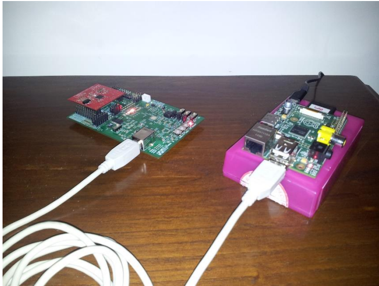
Figure 5.3 - USB connection between coordinator and Raspberry Pi
