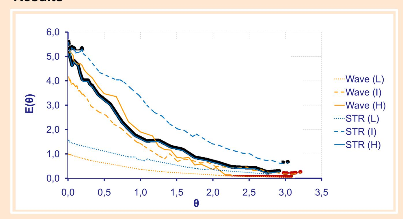
Behavior of Wave reactor at low flow (L) approximates that of the ideal and experimental continuous STR. For the higher flow rates (I and H), behavior of Wave departs from any ideal model.
