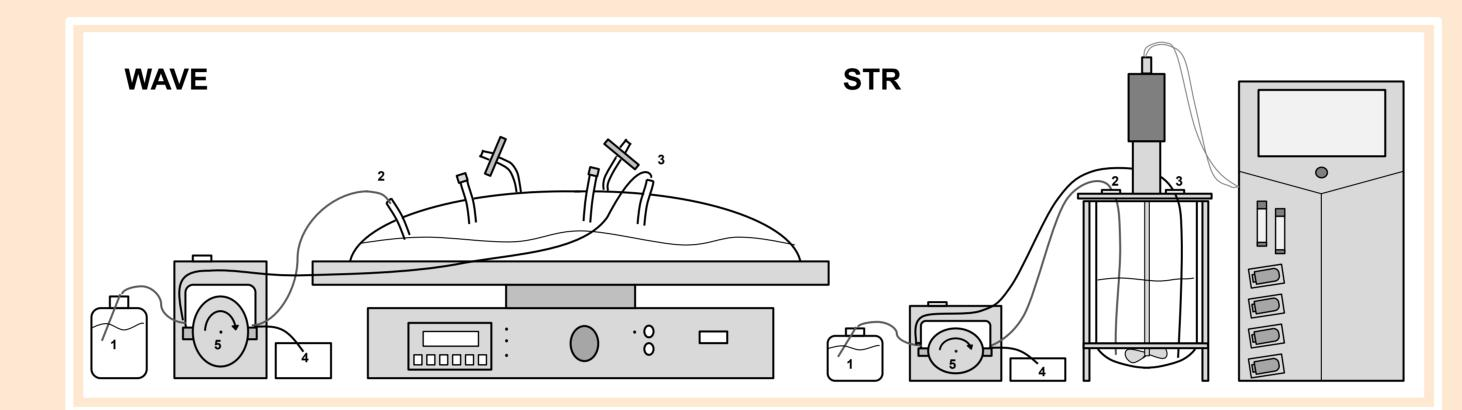
3. Throughout the experiment, samples were taken at the outlet of both reactors, and the samples' absorbance was read at 660 nm.
