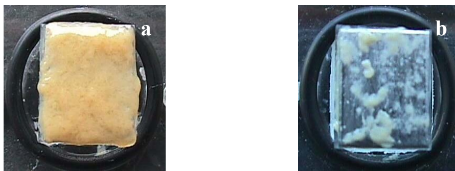
Figure 5.4 Photograph of the coupons with biofilms formed on the stainless steel slides under turbulent (a) and laminar flow (b).
