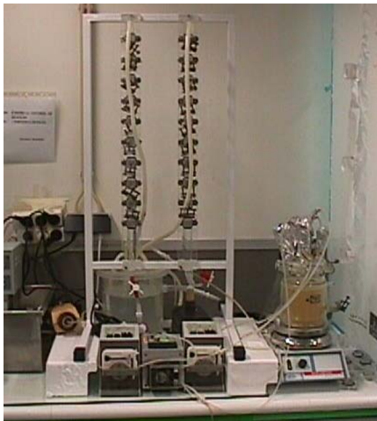
Figure 3.3 Photograph of the flow cell reactor system.
