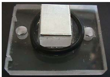
Figure 3.1 Photograph of a piece of Perspex TM with a stainless steel (ASI 316) slide glued.
