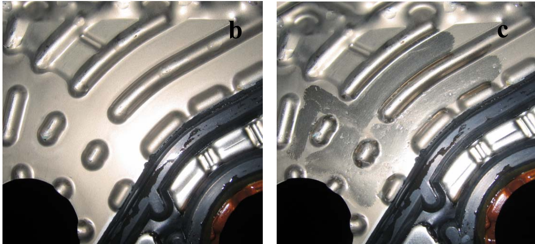
Figure 2.5 Plate heat exchanger (a) where plates were removed for analysis of the biological contaminants. Plate before (b) and after (c) organic deposit removal.
