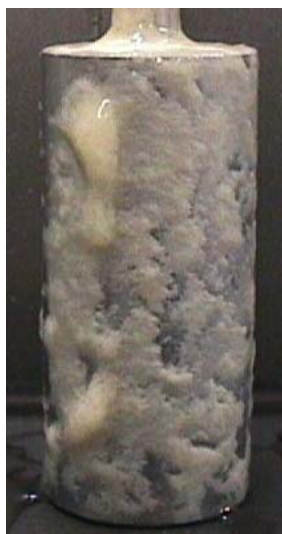
Figure 9.1 Stainless steel cylinder covered with biofilm after 7 d of growth.
