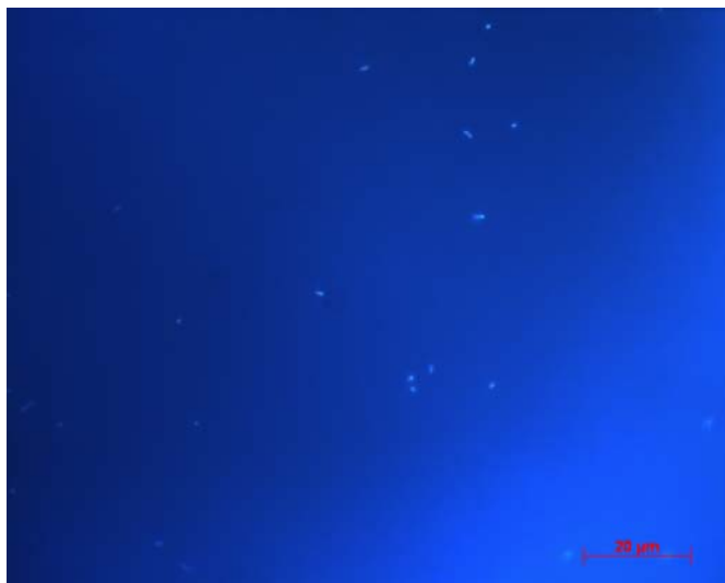
Figure 3.10 Representative microphotograph of a stainless steel surface after the process of scraping and disaggregation of the biofilm. X 1320 magnification, bar =20 \mu\text{m} .
