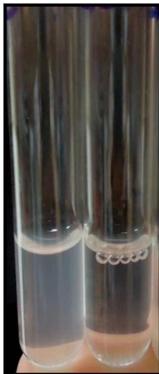
Figure 5. Aspect of coagulation assay using kaolin clay 10 g/L (a model of turbid water) and cMoL (1mg/mL) as coagulant. Left tube represents the control and right tube water treated with cMoL evidencing clarification.
