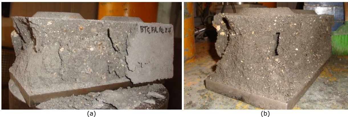
Figure 11 – Failure mode of the CEBs tested under compression: (a) air dry; (b) saturated.
