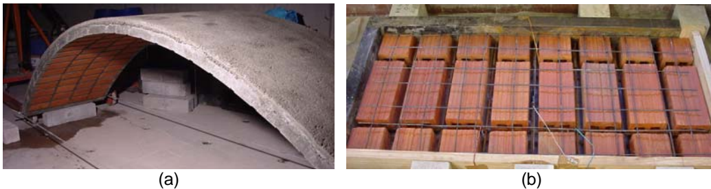
Figure 1 Model of the entire shell (a); detail of the specimen to be tested before the concrete casting (b)
