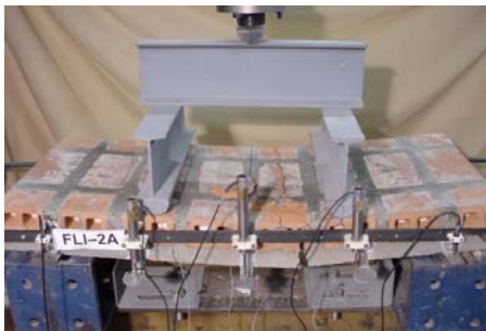
Figure 11 Typical failure mode of panel of series FLI-A
