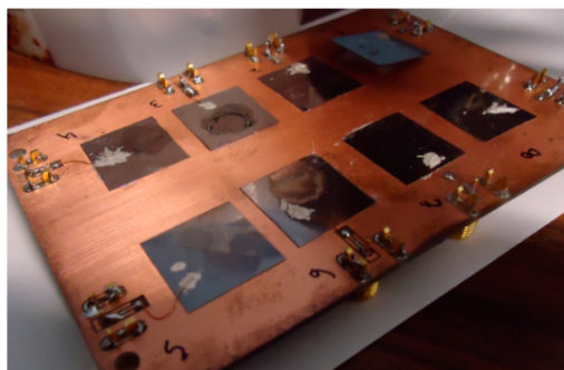
Figure 2. Printed Circuit Board with Radio Frequency (RF) connectors and the 2 \times 2 \text{ cm}^2 \beta -poly(vinylidene fluoride) ( \beta -PVDF) ( 28 \mu\text{m} thickness) transducers, with aluminum electrodes, glued to the Printed Circuit Board (PCB).
