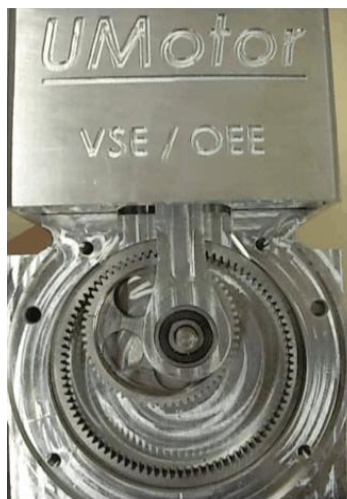
Figure 29 - Hypotrochoid crank system and connecting rod.
