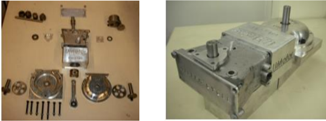
Figure 30 - Exploded view of several parts of the engine and final engine assembly.
