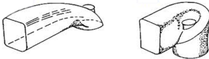
Figure 4 - Direct port (left) and helical port (right).
