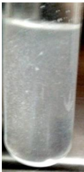
Figure 4.3 – Photography of DODAC:MO(1:2) liposomes prepared by ethanolic injection in citrate-phosphate buffer at pH=9.
