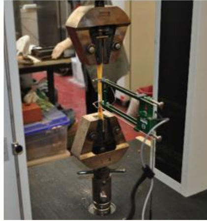
Figure 3-10: Laboratory set-up for epoxy/primer tensile tests.
