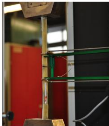
Figure 3-13: Laboratory set-up for GFRP tensile tests.
