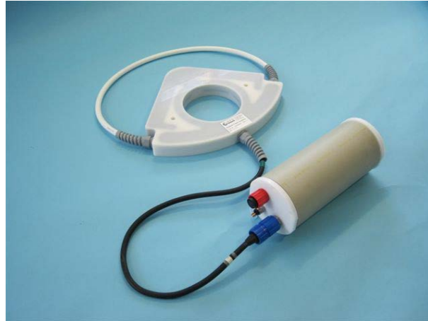
Figure 1.4: SeaText® by WFS, the first commercial RF modem capable to communicate through water and ground [49].
