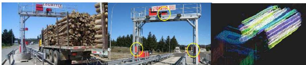
Figura 22 - Logmeter 4000 da Woodtech (Nylinder, Kubénca, & Hultnas)
