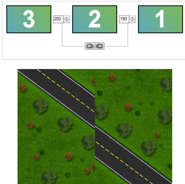
Figure 3.9: Adjusting display bezels with NVIDIA drivers
