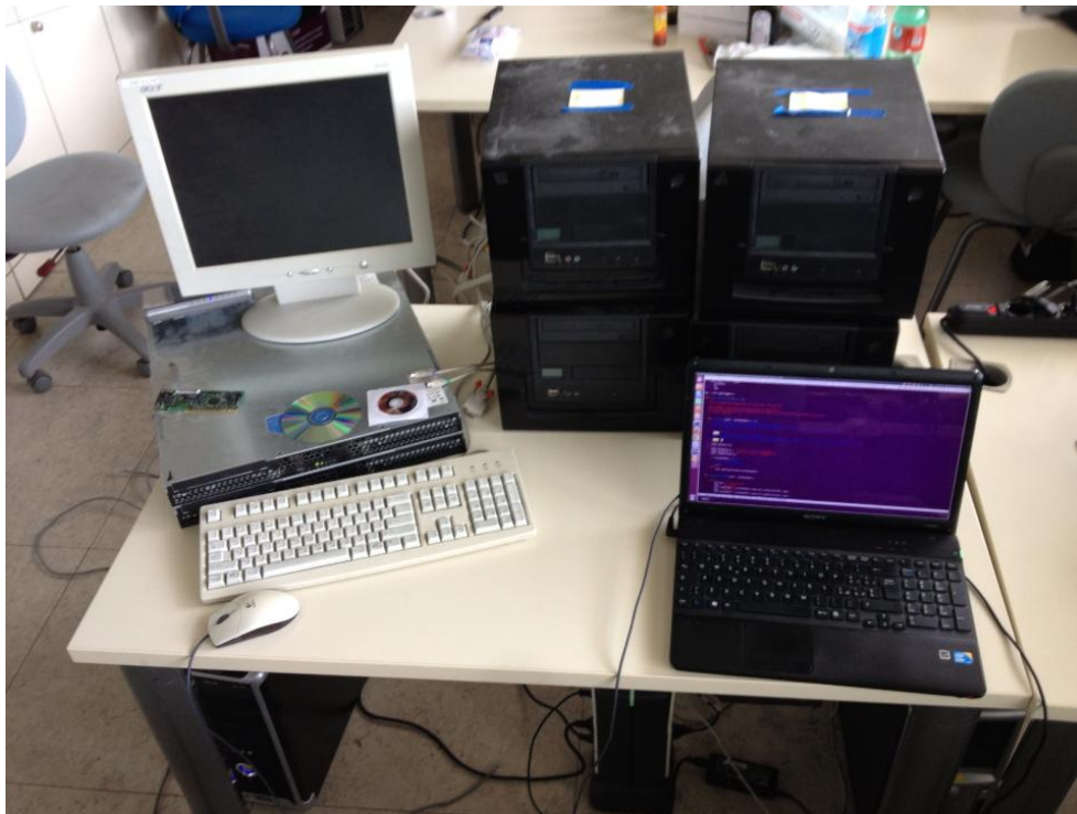
Figure 3.14: Photo of the testing environment. Table : under the monitor - 2 servers; cube computer - aggregation and edge switches; laptop - DC gateway, controller and WEB Platform; Under the table : core switch
